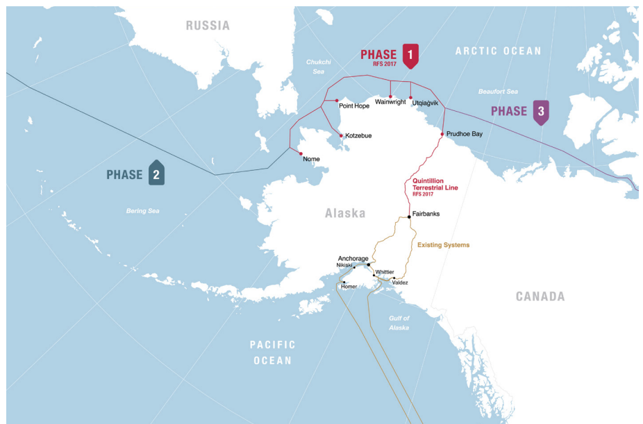
Quintillion is a 1,400-mile subsea and terrestrial fiber optic network that extends over Alaska's North Slope and inland to Fairbanks. Photo Credit: Quintillion
