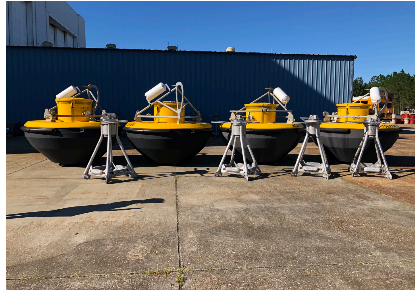
Line of tsunami buoys ready for deployment at the National Data Buoy Center (NDBC) facility in Mississippi.
