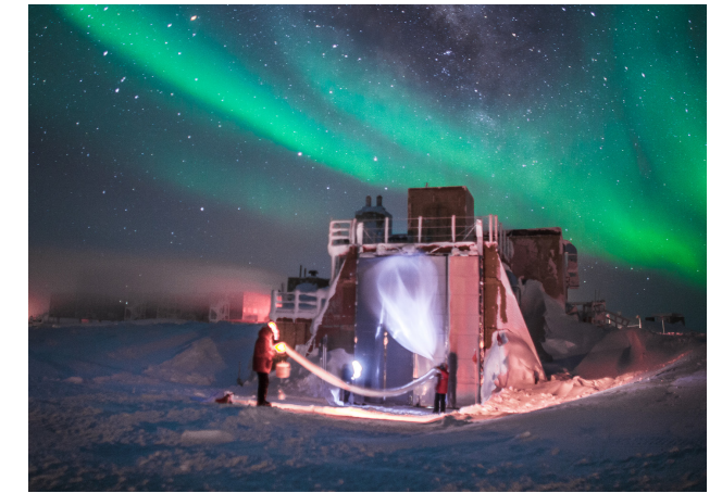
NOAA scientists prepare to launch a balloon that will monitor the thickness of the ozone layer and vertical distribution at the South Pole.
