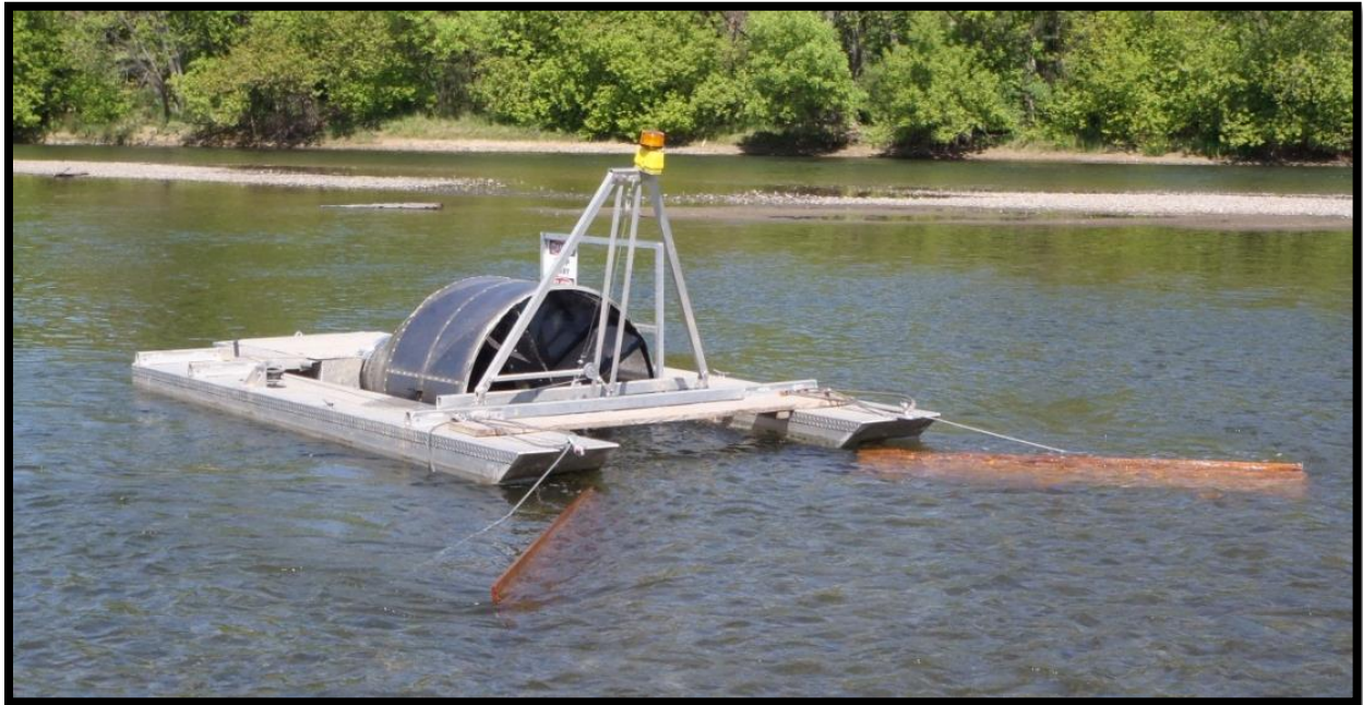
Figure 2: Flow diverters installed on the South Channel rotary screw trap, March 30, 2013.
