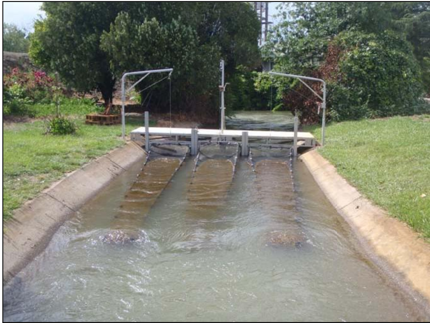
Figure 8. Three fyke nets, sampling platform, and associated apparatus used to sample for fish entrainment in the Portuguese Bend canal.
