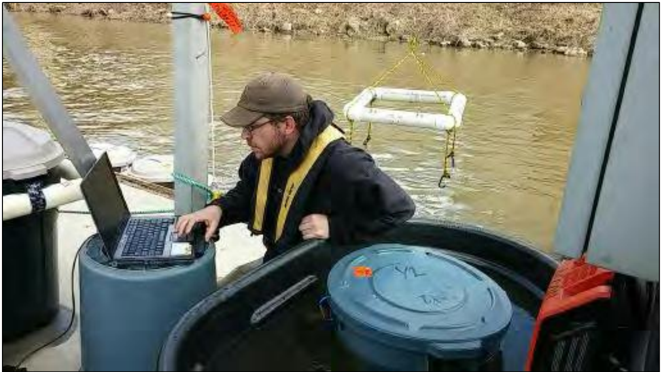
Figure 2-15 Confirming Operation of Acoustic Transmitters before Release
