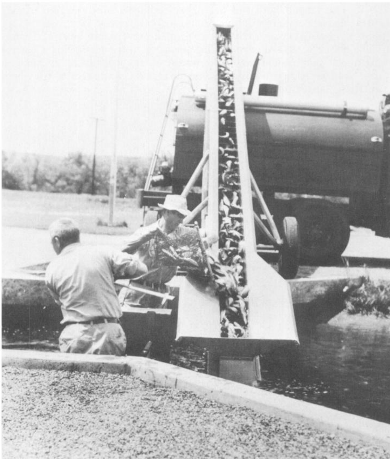
FIGURE 46. Loading trout for planting with a mechanical fish loader, San Joaquin Hatchery. Photograph by William M. Carah, May 1956.
