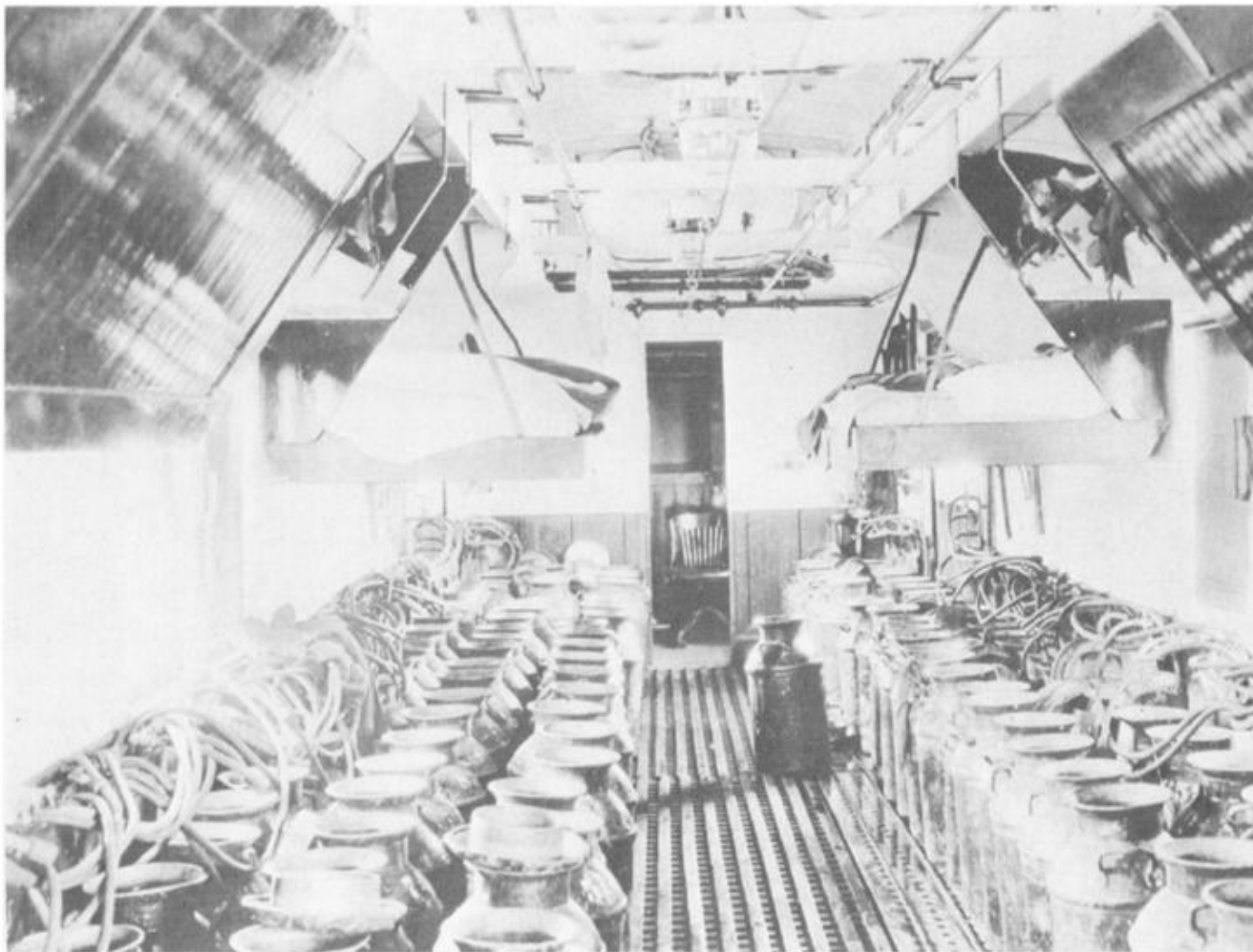
FIGURE 29. Interior of railroad fish distribution car. Hoses supplied air to the cans containing fish. Bunk beds provided sleeping accommodations for crew members.
