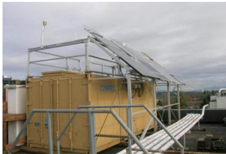
Figure 2-2. PV module and equipment deployment at the University of Oregon, Eugene, Oregon
