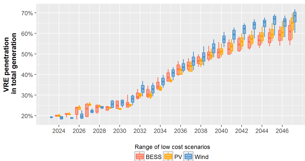
Figure ES-2 Range of VRE penetration in total generation in each model year in the BESS, solar PV, and wind technology cost scenarios
