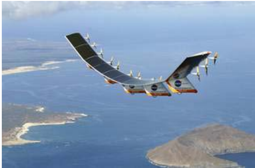
Figure 1. Project Helios solar-powered electric aircraft.
