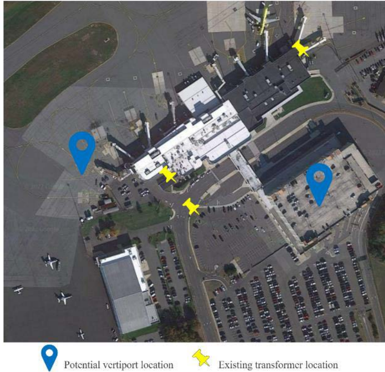
Figure 11. Atlantic City International Airport Transformer and Potential Vertiport Locations.
