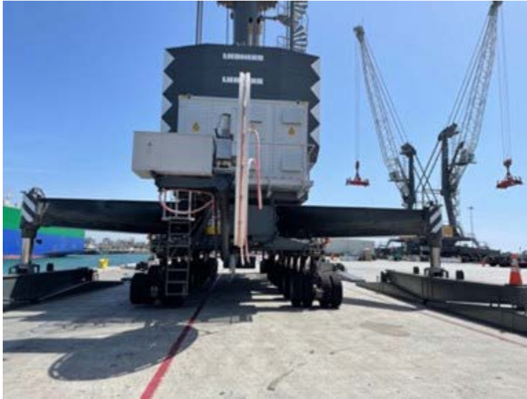
Figure 32. Q1 2022: Liebherr 420 Hybrid-Electric Crane
