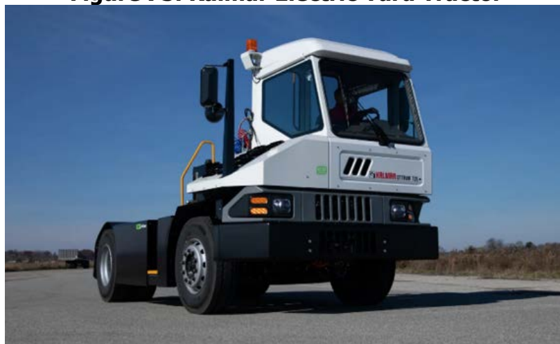
Figure 75. Kalmar Electric Yard Tractor
