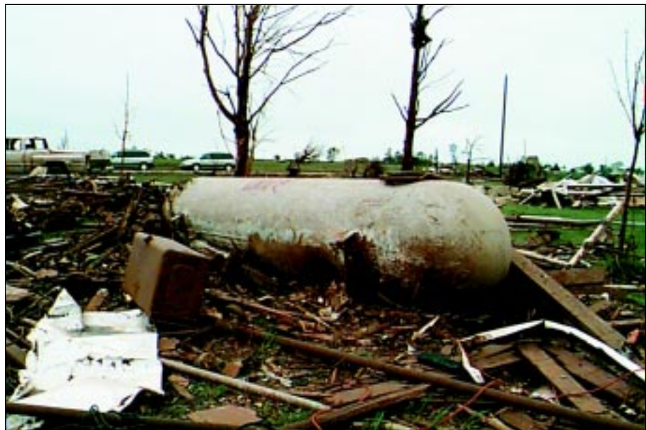
FIGURE 3-23: Wind displaced this very large propane tank in Bridge Creek, Oklahoma; its original location could not be determined. This area was hit by the vortex of a violent tornado.
