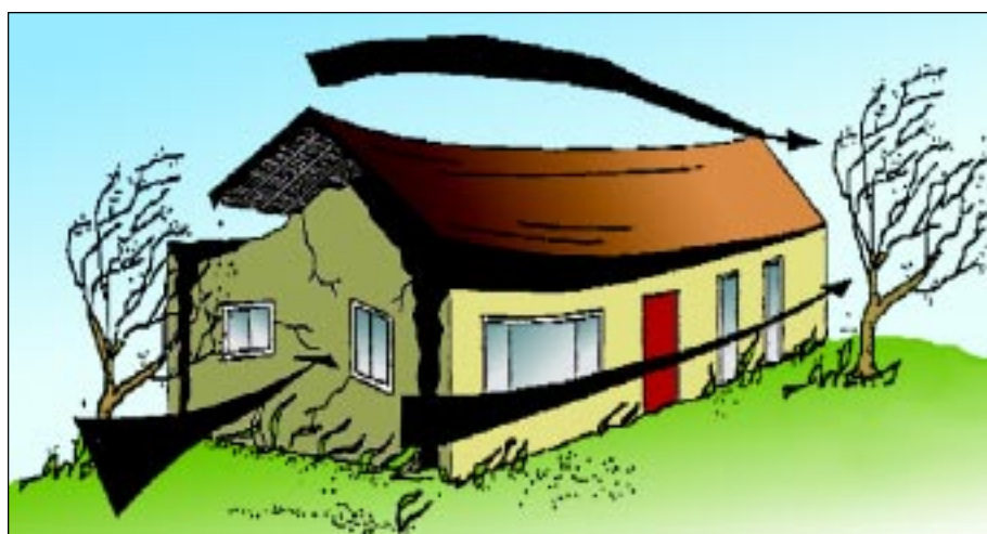
FIGURE 3-4: This building failure is the result of inward wind forces and uplift wind forces acting on a building during a high wind event.
