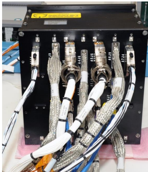
Figure 10-2. The Command and Telemetry Processor (CTP)
