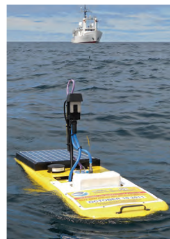
NOAA's autonomous Wave Glider harnesses wave energy to propel itself across the ocean surface. Solar-powered monitoring equipment collects information about pH and carbon chemistry
