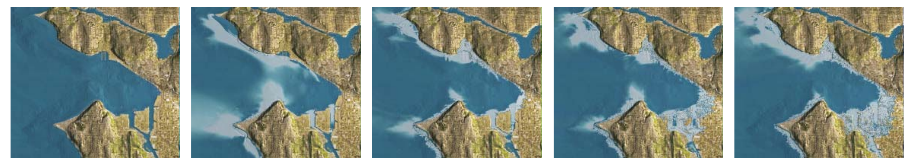
Figure 3. Freeze frames of animation of modeled tsunami at 30-second intervals (from left to right). The wave crest is colored pale blue. Note that because Harbor Island is uplifted by the earthquake, the Duwamish Waterway initially drains rapidly before the wave reflects off the north side of the bay and then inundates the Harbor Island area.
