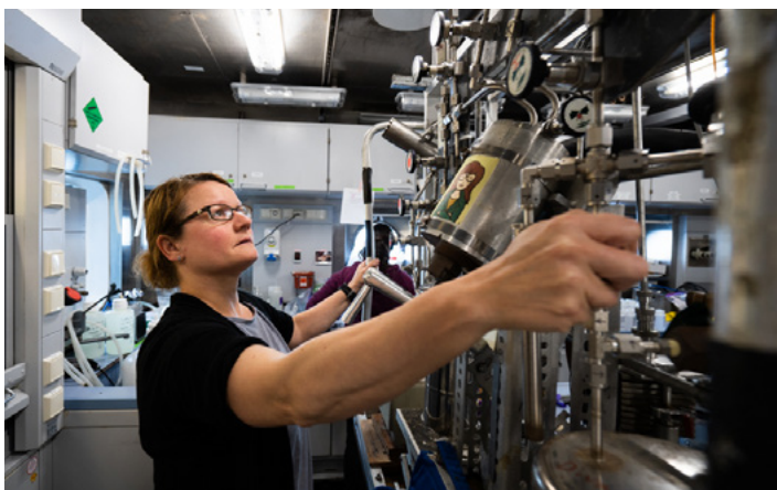
(Top) The crew of the catcher-processor Starbound posing with a pop-up float prior to deployment. These were among the first industry collaborators to deploy these floats in the Bering Sea in August 2020. Credit Starbound Crew; (Bottom) Research Scientist Tamara Baumberger (Oregon State University/NOAA PMEL) extracting methane samples from a gas tight sampler onboard R/V Falkor to better understand how and why methane seeps on the seafloor off the U.S. Pacific Coast have formed. Credit Shelton Du Preez/Schmidt Ocean Institute
