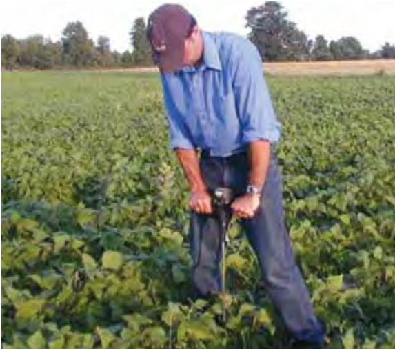
Figure 23.1. A soil penetrometer is a useful tool to assess soil compaction. Measurements are best made when soils are moist and friable (around field capacity).
