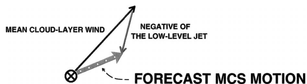
FIG. 1. Schematic of the original vector technique, with MCS core motion (thick dotted arrow) expressed as the vector sum of 1) advection of cells by the mean cloud-layer wind (arrow pointing to upper right) and 2) cell propagation directed into the low-level jet (arrow pointing to bottom of page). MCS centroid is depicted by the cross symbol (after Corfidi et al. 1996).
