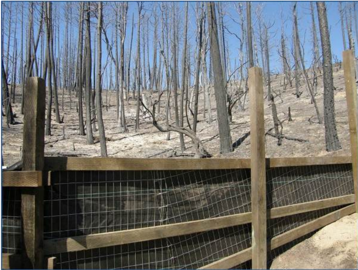
Figure ES-4. This photograph shows a closer view (compared to Figure ES-3) of a control site looking upslope from the downslope side of its sediment fence. Note the relatively uniform nature of the soil surface which is covered by ash, the remnant dead trees evident throughout the burned swale and that there is no obvious stream channelization in the swale prior to the occurrence of post-wildfire rain. Because it is a control site, the swale was not salvage-logged nor contour subsoiled and was disturbed only by the Ponderosa Fire itself. Although undisturbed by any post-wildfire treatment, the control sites produced the highest water runoff and average soil erosion over the first winter season (see Figures ES-7 and ES-8).
