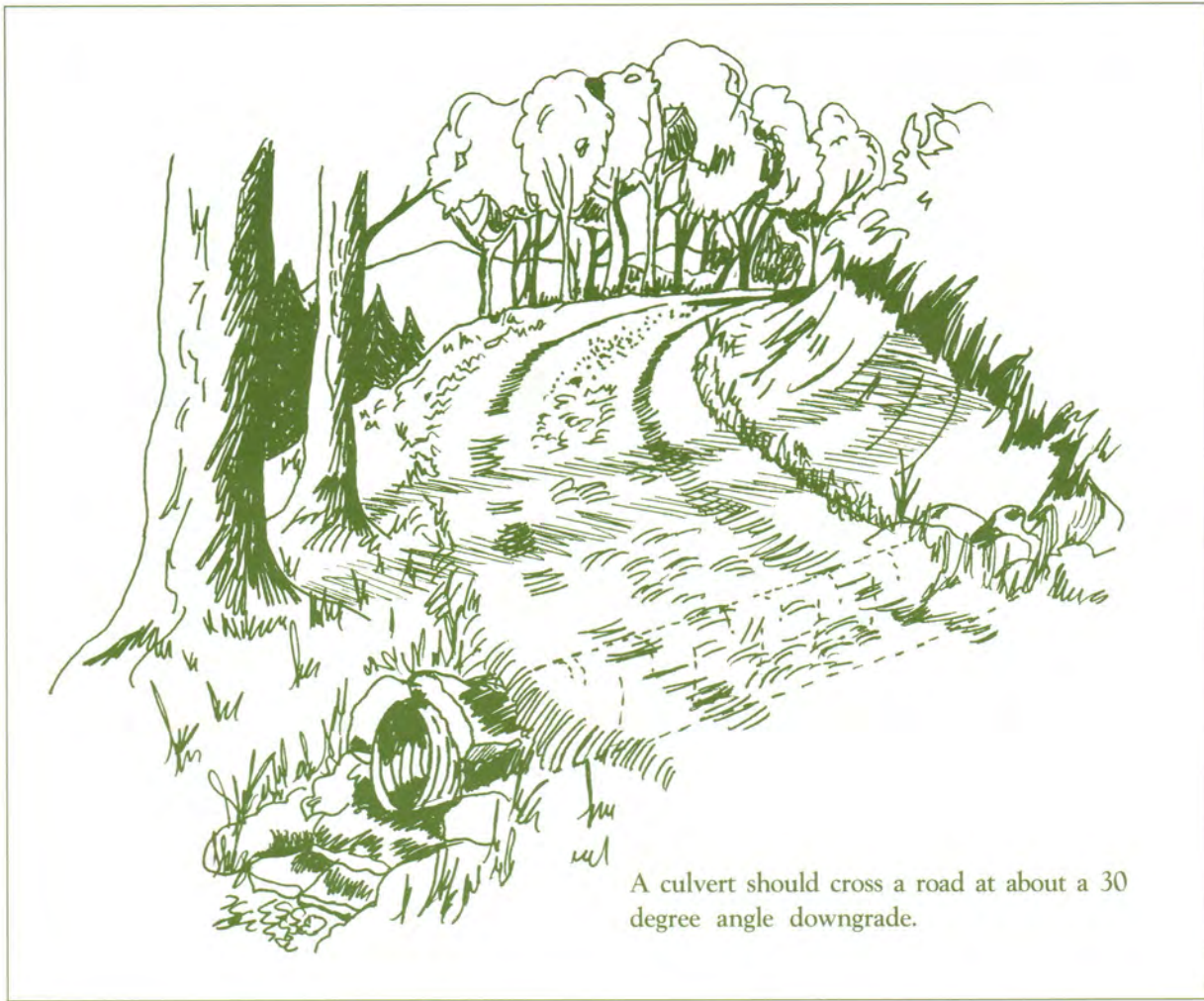
FIGURE 3 CULVERT INSTALLATION (GEORGIA FORESTRY COMMISSION 1988)
