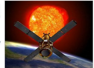
The Reuven Ramaty High Energy Solar Spectroscopic Imager (RHESI), launched in 2002, explores the explosive energy released in solar flares. (Source: NASA)
