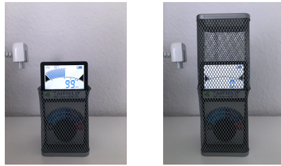
FIG. 1. Electric field measurement with and without Faraday shielding.
