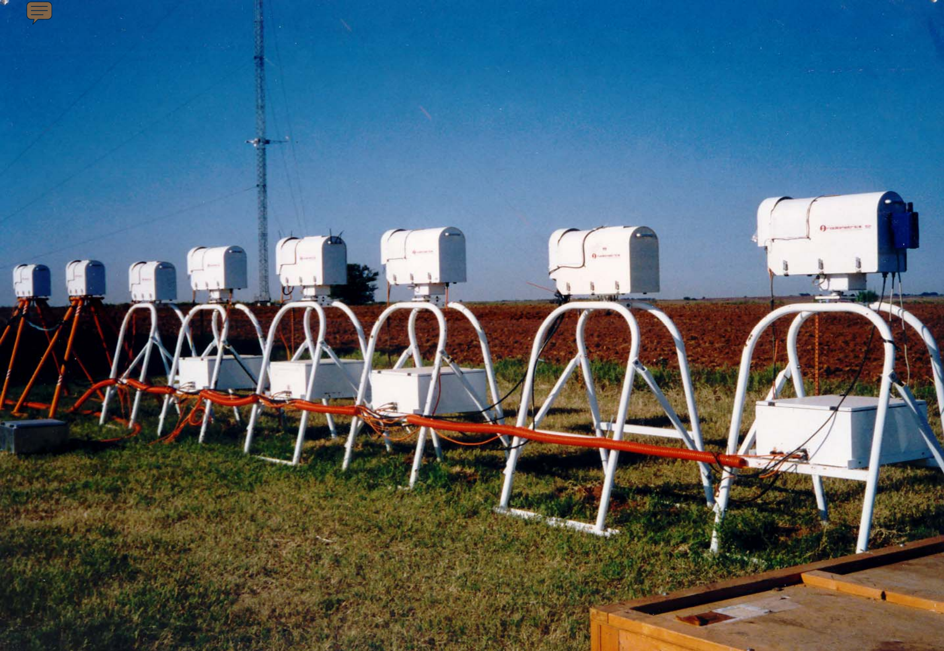
DOE ARM radiometers calibrate radiosondes for climate research.
