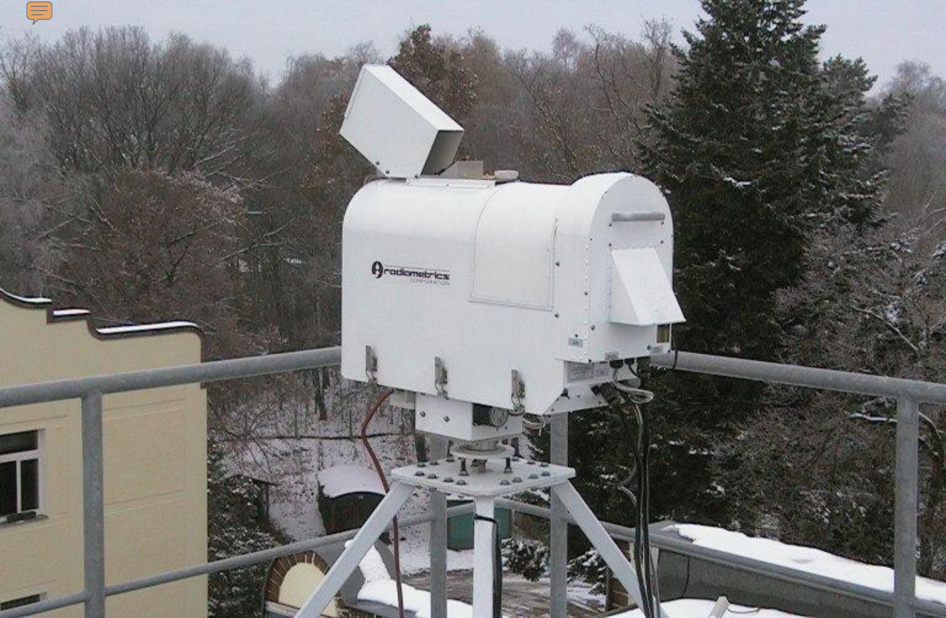
German Weather Service radiometer and 6-hr radiosonde comparisons since 1998 [Güldner and Spänkuch, JAOT , 2001]
