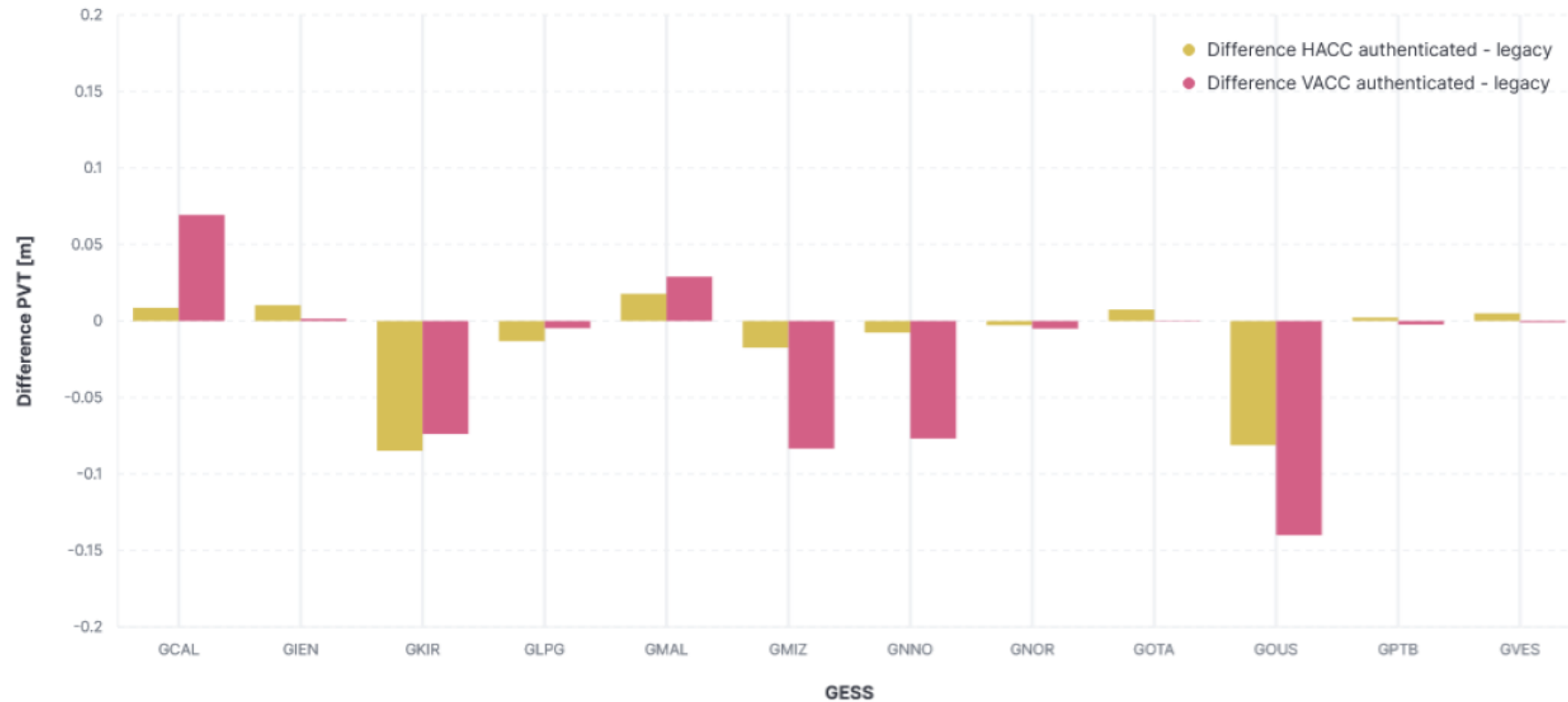
Average difference between legacy and OSNMA vertical and horizontal position accuracy (95%) measured at each TGVPx GESS from 1 st May until 30 th June 2022
