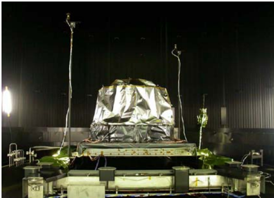
Thermal Vacuum Test of L-band Antenna Engineering Model (February 2007) 【MEXT】
