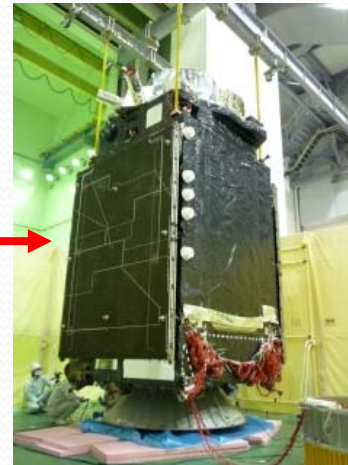
Separation Shock Test (1.13/2010-1.14/2010)
