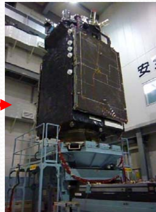
Sine Vibration Test (7/12/2009-6/1/2010)
