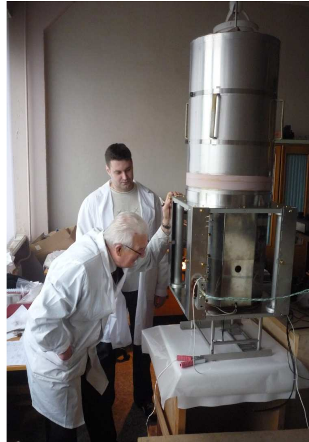
Assembling of the fountain mainframe & magnetic shield
