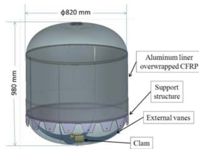
Fig.-9 Concept of CFRP propellant tank
