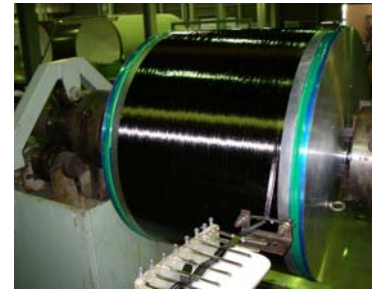
Fig.-10 CFRP overwrapping test
