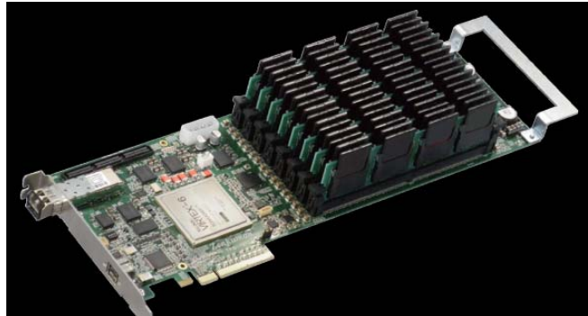
Fig.-3 The FPGA board manufactured by Technoscope which can analyze 32 4K4K-frames with 40 seconds.
