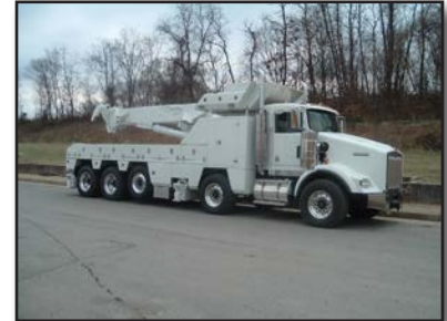
Figure 8.8 – Large wreckers may be required to remove large vehicles from the roadway.
