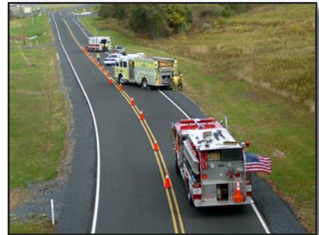
Figure 7.3 – Use emergency vehicles to block incident activities from approaching traffic. (Photo/Bob Esposito, Pennsburg, Pennsylvania)
