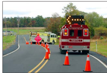
Figure 7.30 – Some fire apparatus are equipped with lighted directional arrow or message signs. (Photo/Bob Esposito, Pennsylvania)
