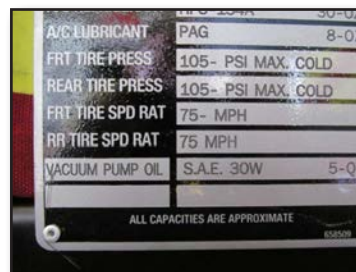
Figure 7.10 – Post the speed limit on the dashboard or a plate elsewhere in the cab near the driver seat. (Photo/Mike Wieder)
