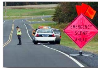
Figure 7.18 – Temporary traffic control signs should be pink in color. (Photo/Bob Esposito, Pennsburg, Pennsylvania)
