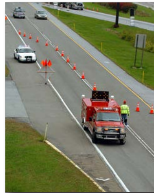
Figure 7.17 – Traffic cones assist in guiding motorists away from the incident area. (Photo/Bob Esposito, Pennsburg, Pennsylvania)
