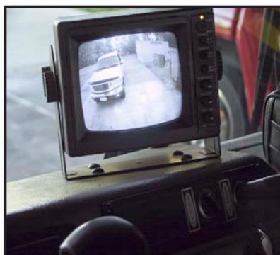
Figure 3.19 — The image captured by the rearview camera is displayed on a monitor inside the cab. (Photo/Mike Wieder)
