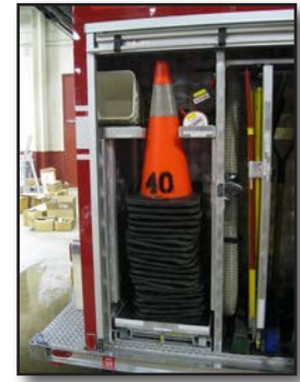
Figure 7.26 – There are many locations on a vehicle for storage of traffic cones. (Photo/Mike Wieder)
