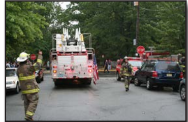
Figure 7.12 – Use at least one backer when the apparatus is being moved in reverse. (Photo/Ron Jeffers, Union City, New Jersey)
