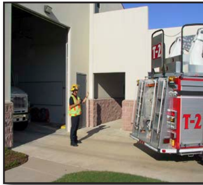
Figure 3.17 — Always use at least one backer when operating the vehicle in reverse. (Photo/Mike Wieder)
