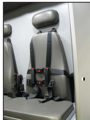
Figure 7.9 – Use ambulance restraint systems when provided. (Photo/Mike Wieder)
