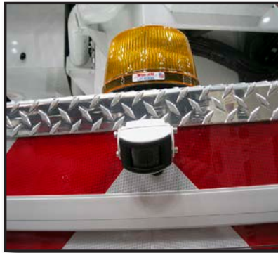
Figure 3.18 — Many apparatus are equipped with rearview cameras. (Photo/Mike Wieder)
