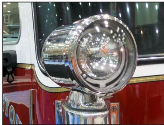
Figure 4.20 – An oscillating warning light. (Photo/Mike Wieder)
