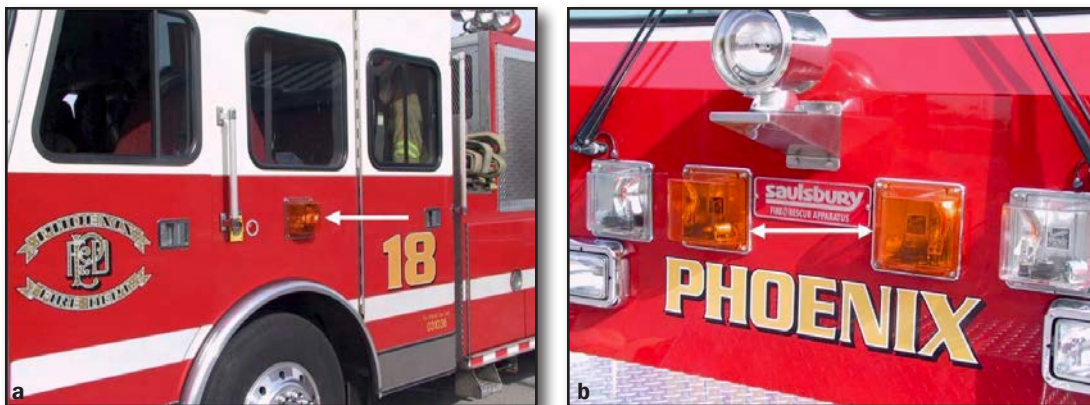
Figures 4.22a and 4.22b – Amber lights may be positioned around the vehicle. (Photo/Mike Wieder)
