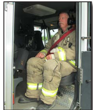
Figure 7.14 – Occupants must be seated and belted when the vehicle is in motion. (Photo/Mike Wieder)
