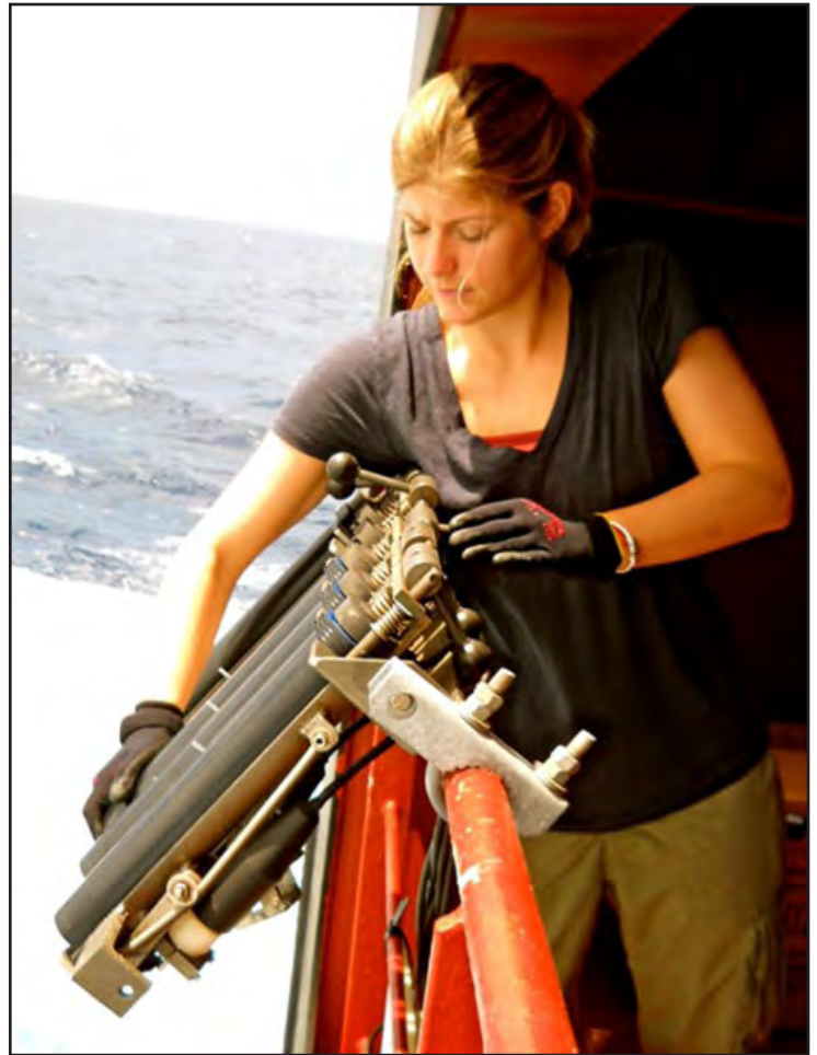
Jessica Raymond loading the XBT Launcher. Photo: courtesy of Scripps
