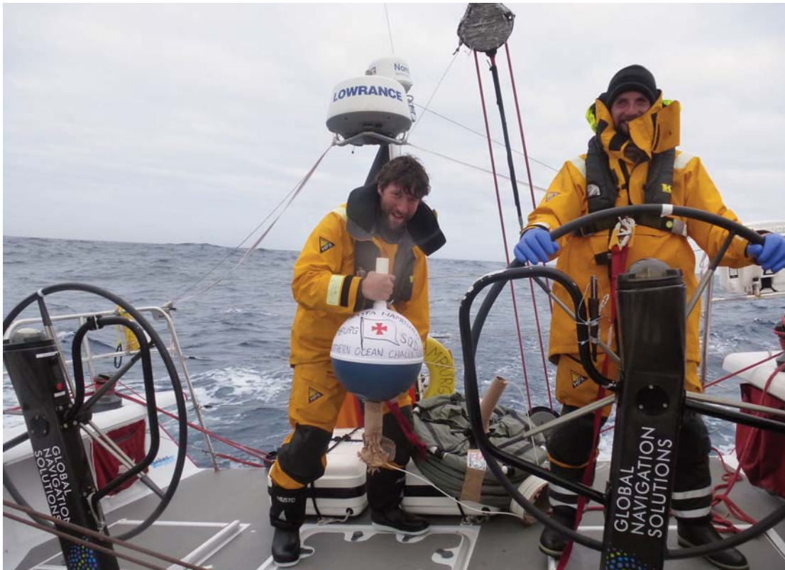
HASPA HAMBURG watch captain Felix Zahn deploys a NOAA drifter in the Southern Ocean; at the helm: Vincent Weide
