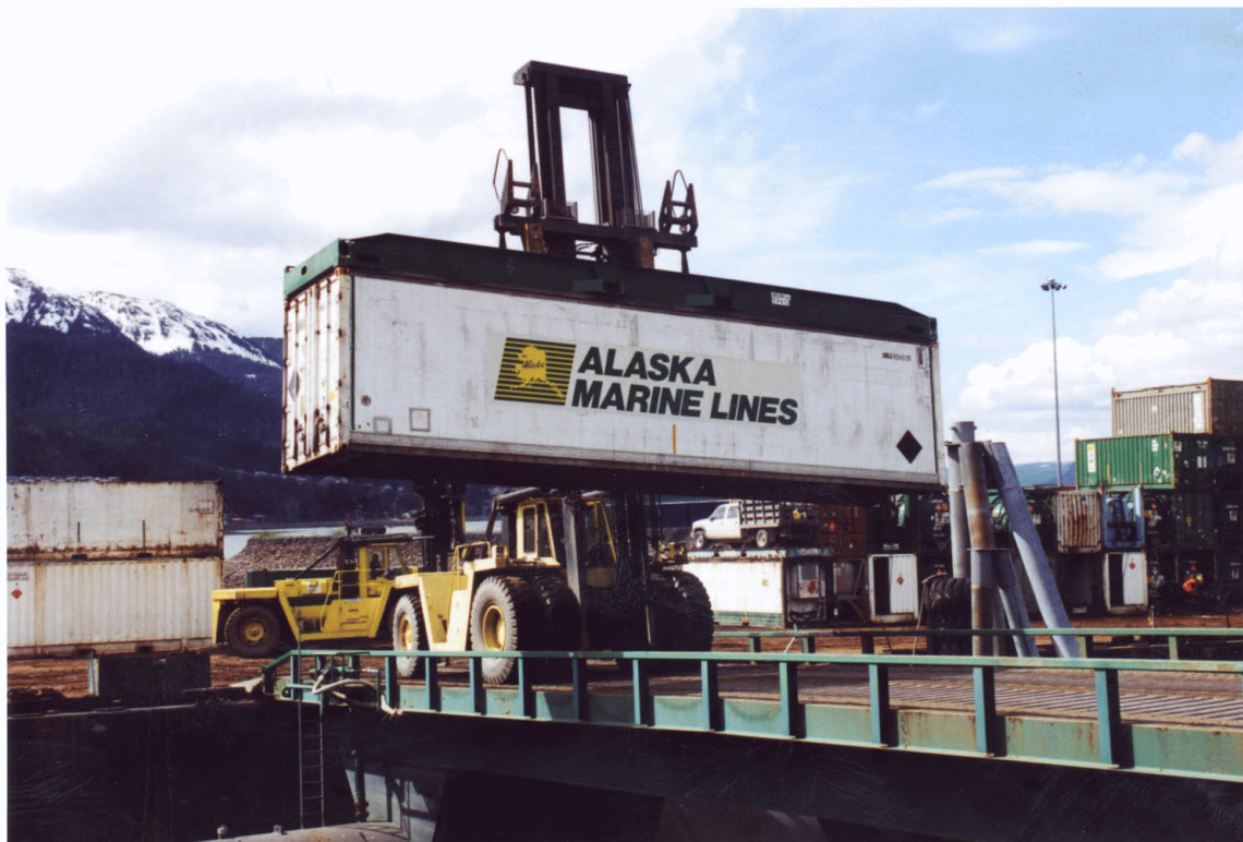
Figure 4. Unloading containers from the Nana Provider at the dock in Juneau
