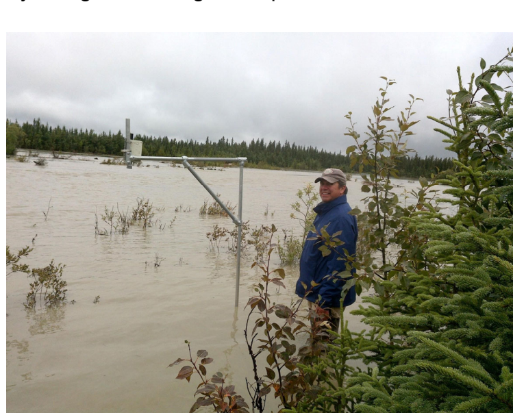
Figure 10: Fairbanks WFO Electronics Technician Keith Flewellen standing next to a temporary igage deployed to a flooded area on the Delta River. The igage measures distance to the water and transmits the data via Iridium satellite. A small solar panel and battery make the system self contained.
