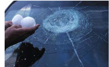
2"-2 1/2" hail causing severe damage
