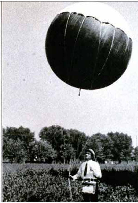
Sending up a sounding balloon: The parachute wafts the basket of instruments gently to the ground after the balloon bursts.
