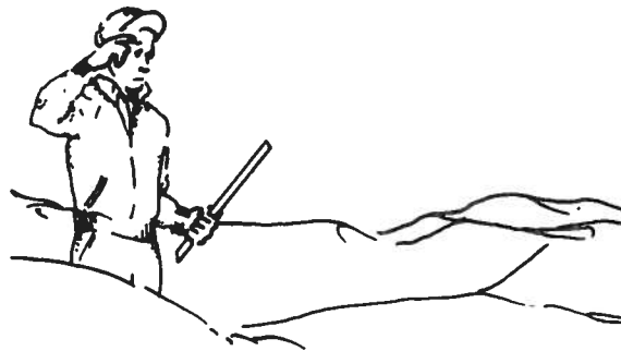
2. Measure each new snow. Use good judgment in selecting spots where the snow is least affected by drifting.
