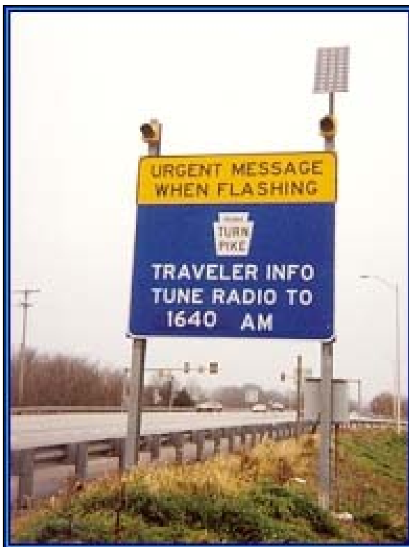
Figure 1. A Highway Advisory Radio Station along the Pennsylvania Turnpike in the western Philadelphia suburbs. Such roadside signs alert drivers to listen to a radio station to receive urgent travel information. Highway Advisory Radio systems can be programmed to broadcast NWS weather information heard on NOAA Weather Radio (NWR).
