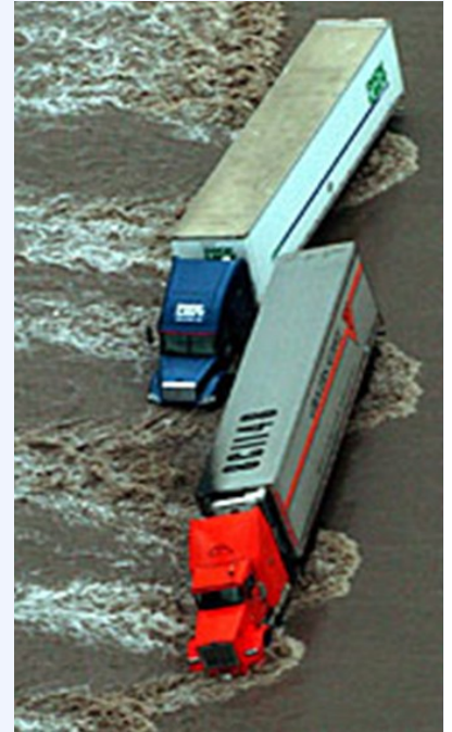
Semi-trailer trucks being floated. Note that the water comes up only to the wheel wells!
