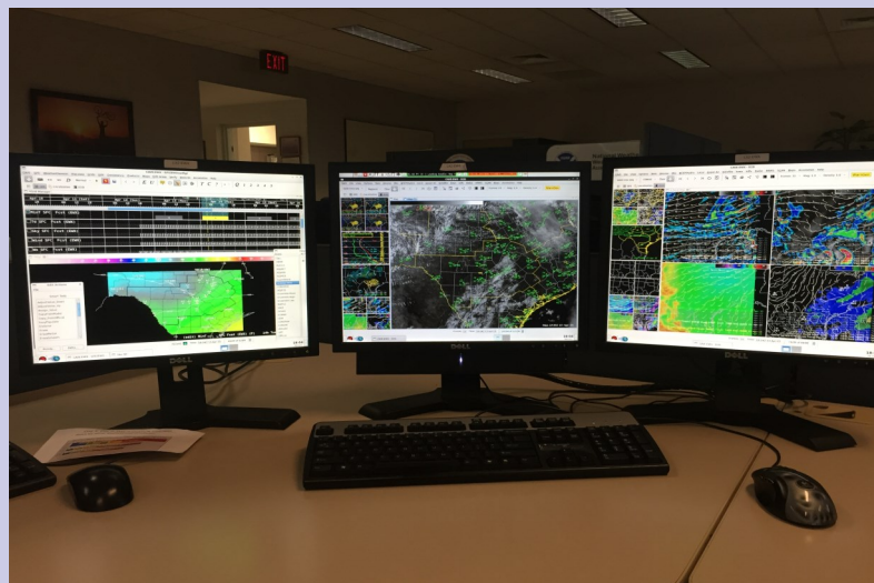
AWIPS2 Workstation at EWX office
