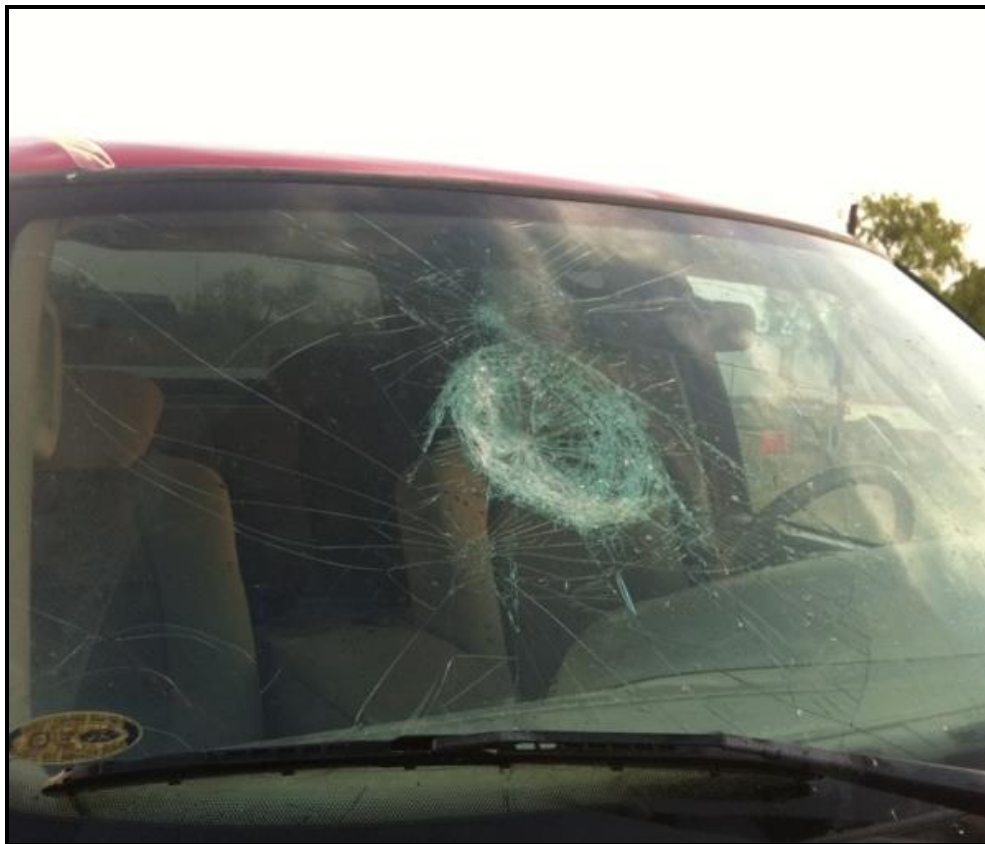
Figure 5. Hail damage 6 miles NNW Crystal City, TX, on March 31, 2013.
