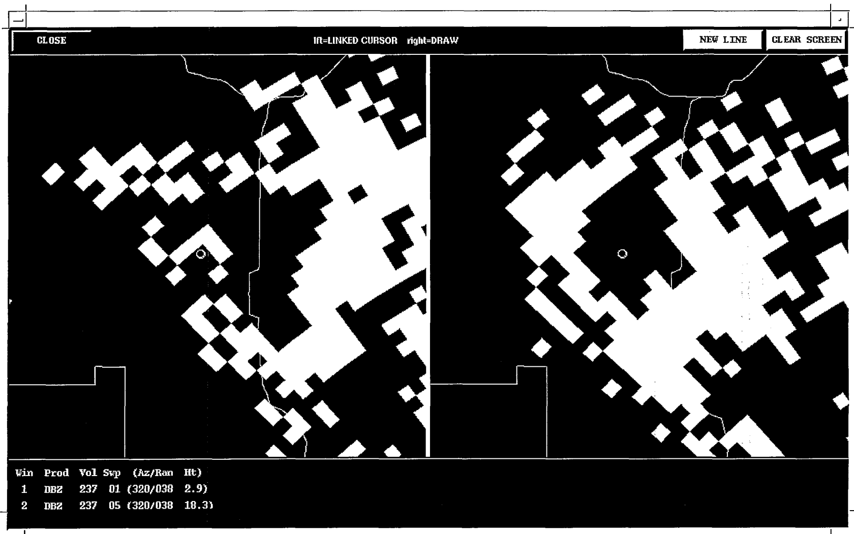
Fig. 7. (A) shows evidence of a hook echo (>55 dBZ) to the northwest of the reference marker at an elevation of 970 m AGL. The positions of the main downdraft regions are shown northwest of the white circle and across an area from the north-northeast through southeast. (B) shows greater reflectivity, at an elevation of 6100 m, surrounding the reference marker. A reflectivity v-notch is also shown on the southeast flank of the storm.
