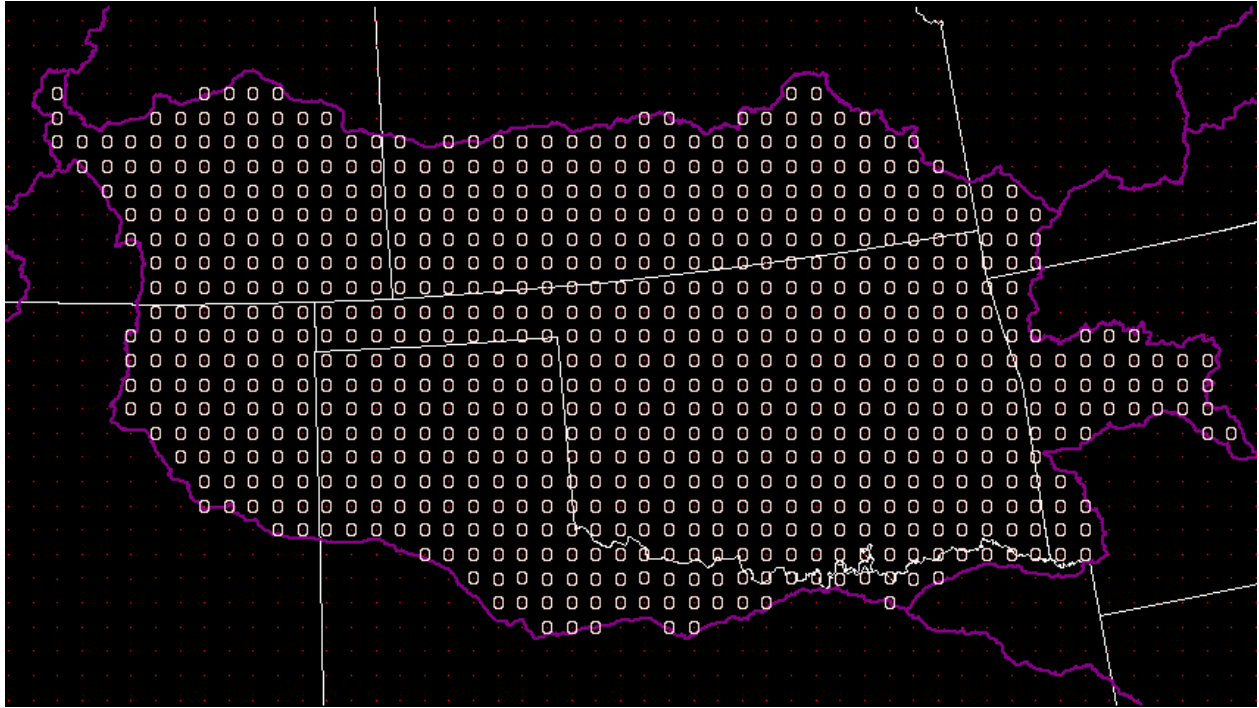
Figure 4. 30-km verification grid shown for the ABRFC area, where gridpoints within the bounded RFC service area are circled.
