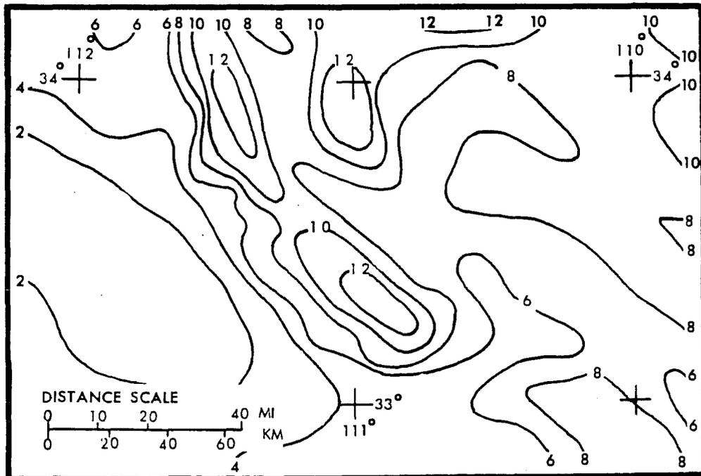
Figure 3.3.--A first approximation to the orographic PMP (inches) for 10 mi<sup>2</sup> (26 km<sup>2</sup>) 24 hr in southeast Arizona.
