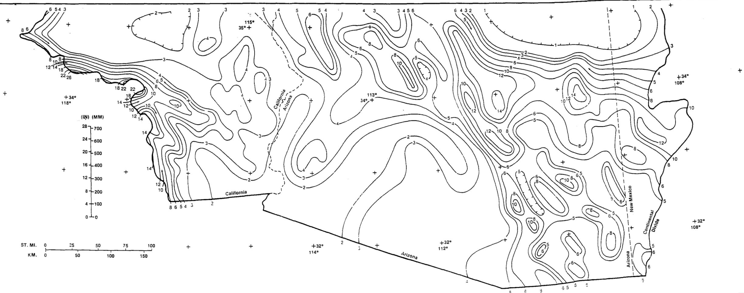
FIGURE 3.11d (Revised) — 10-mi<sup>2</sup> (26-km<sup>2</sup>) 24-hr orographic PMP index map (inches), southern section.
