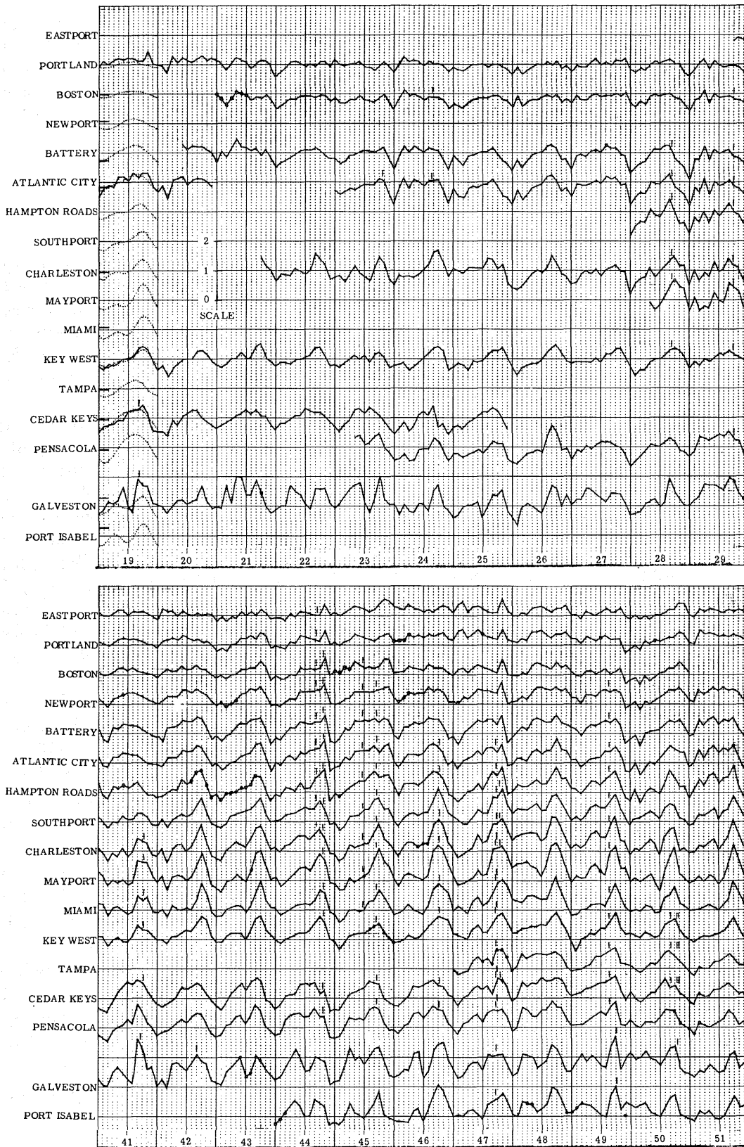
FIGURE 0.3.—Monthly mean sea level at selected Coast and Geodetic Survey tide stations, 1919–1961. The normal monthly means included in the official tide predictions are shown as dashed lines along with the observed values
