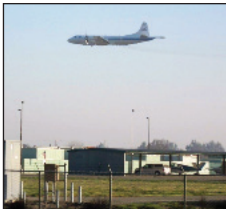
The NASA P-3B made low approaches at local airports during this mission, getting as low as 100 feet to make key air quality measurements.
