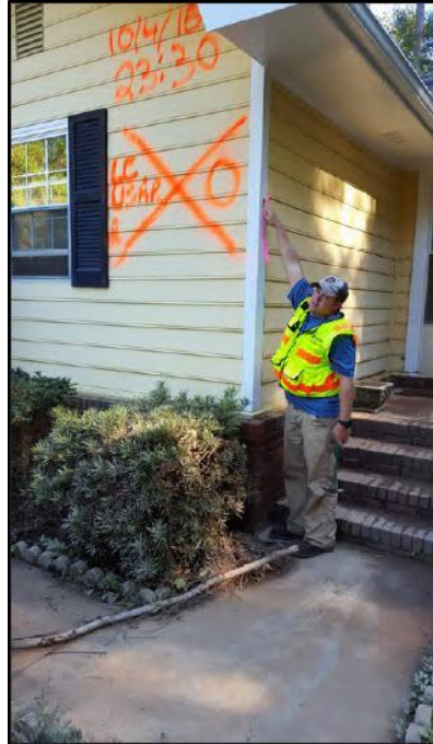
Figure 7: U.S. Geological Survey measures high water at flooded home in Lexington County, SC for the October 2015 flood. Source: USGS
