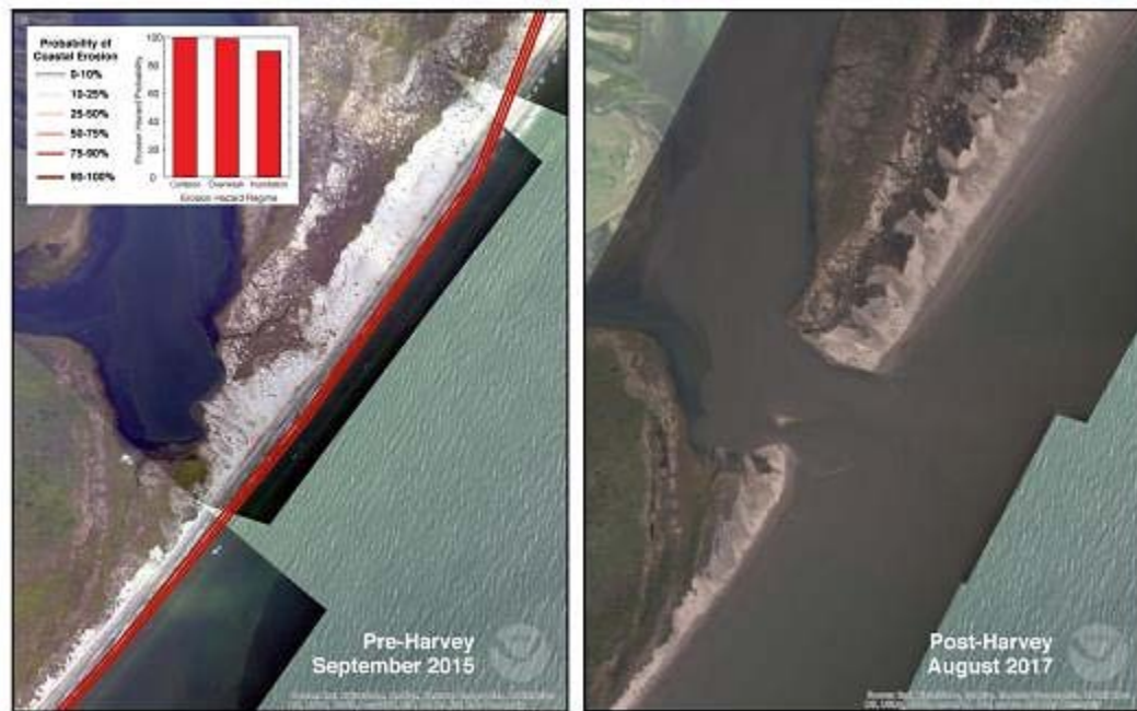
Figure 15: Large 340 meter-long breach at the north end of Matagorda Island produced by storm surge and wave action during Hurricane Harvey. Source: USGS/NOAA Hurricane Harvey photo comparisons
