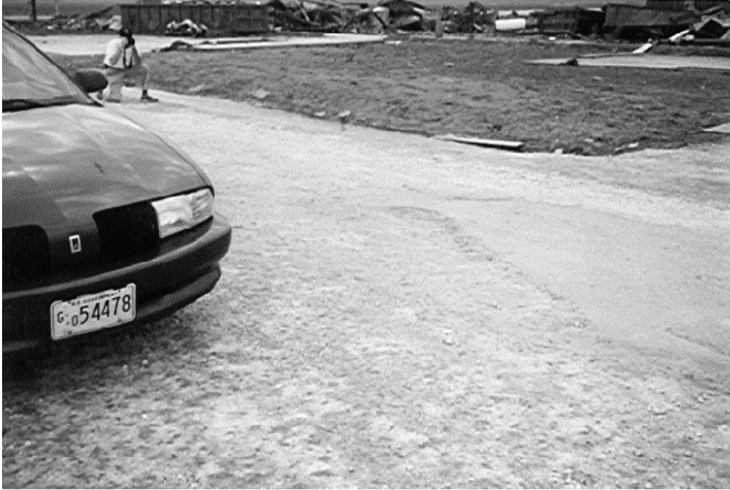
Asphalt stripped from the road by the Jarrell tornado in the Double Creek Estates subdivision. Photograph by I. Hakkarinen, NOAA/NWS.
