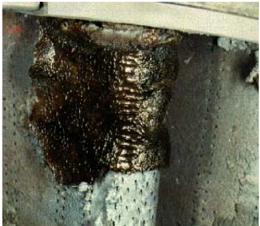
Figure 2. Damage to this jet turbine resulted from ingesting volcanic ash. The ash melted and formed an acidic glass-like coating on the engine.
